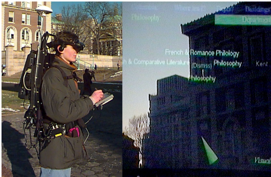
The MARS (Mobile Augmented Reality System), the first outdoor mobile AR system[1]
